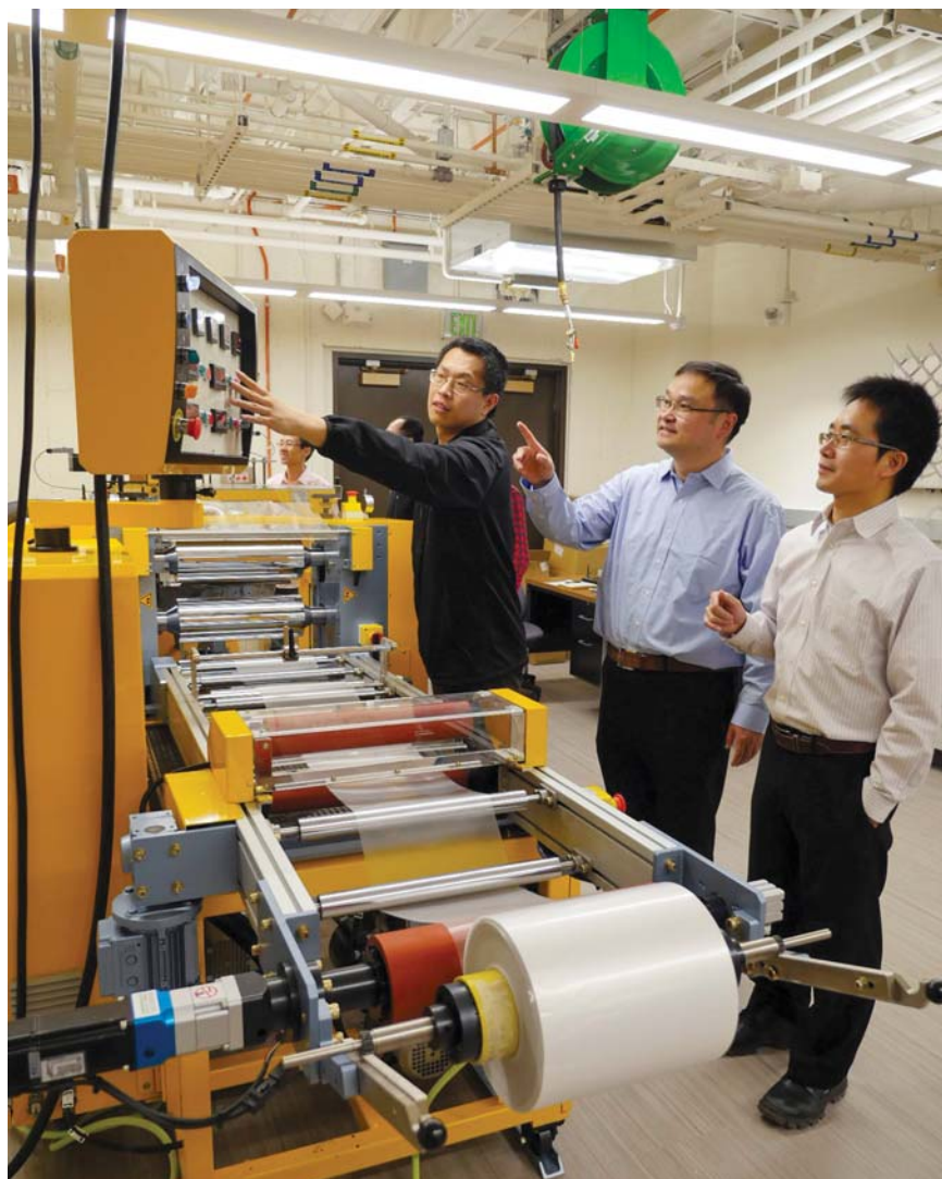
FIGURE 1. YAOGUANG MA, XIAOBO YIN, AND RONGGUI YANG (left to right) oversee the roll-to-roll production of the glass-polymer film used in their radiative cooling experiments.
