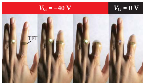
FIGURE 3. FINGER FILMS. A stretchable, polymer-based thin-film transistor (TFT) worn on the knuckle of an index finger is used to control an LED on the middle finger. The transistor switches on when a sufficiently large gate voltage V_G is applied, remains on as the finger flexes, and switches off when the gate voltage is turned off. (Photo credit: Jie Xu and Sihong Wang of Zhenan Bao's group at Stanford University.)
