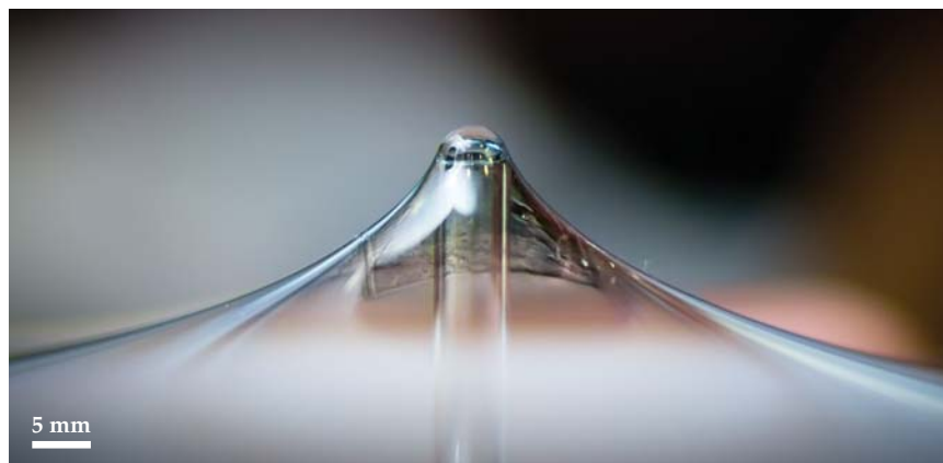
FIGURE 1. A POLYMER TRANSISTOR , visible as a 20-mm-wide translucent patch in the film pictured here, is resilient to stretching, twisting, and poking. (Photo credit: Amir Foudeh, Jie Xu, and Sihong Wang of Zhenan Bao's group at Stanford University.)
