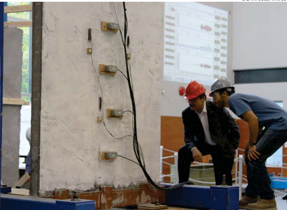
A FULL-SCALE WALL , 3 m tall by 2 m wide, is mounted on a shake table for testing. After applying shaking patterns derived from actual earthquakes, Nemkumar Banthia (left) and Salman Soleimani will examine the wall for cracks and other damage. This wall has a 1-cm-thick coating of eco-friendly ductile cementitious composite.
