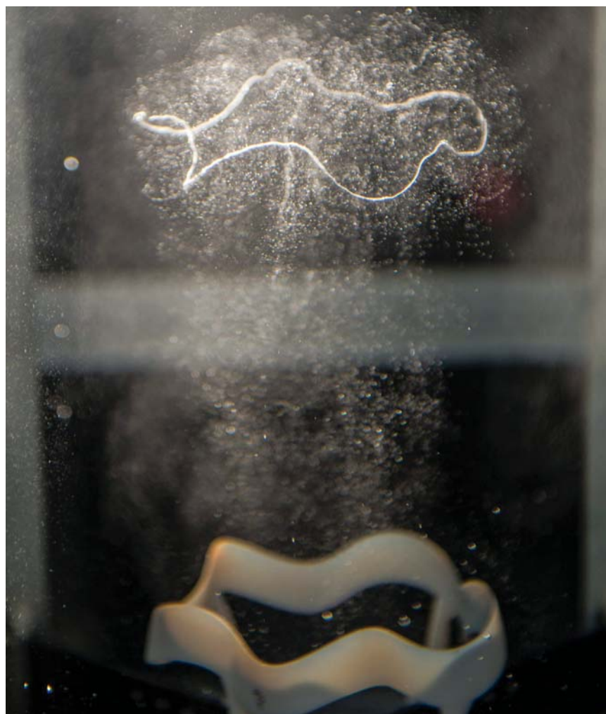
FIGURE 1. A VORTEX RING (top) was generated by the swift downward acceleration of a ring-shaped hydrofoil (bottom), roughly 10 cm in diameter, in a tank of water. The coils in the vortex ring are indicative of a topological property known as helicity. (Image courtesy of William Irvine.)
