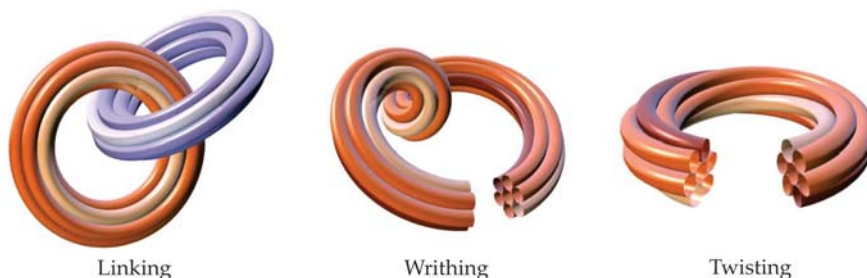
FIGURE 2. HELICITY describes how long, thin flow structures known as filaments (orange and purple) wrap around one another. In vortex rings, those filaments bundle in tubes, and helicity can therefore take three forms: Pairs of tubes can interlock (linking), a single tube can coil around on itself (writhing), and individual filaments can wind around the tube's centerline (twisting). The writhing and twisting forms are interconvertible but can't be converted to linking without breaking and reconnecting filaments. (Adapted from ref. 1.)
