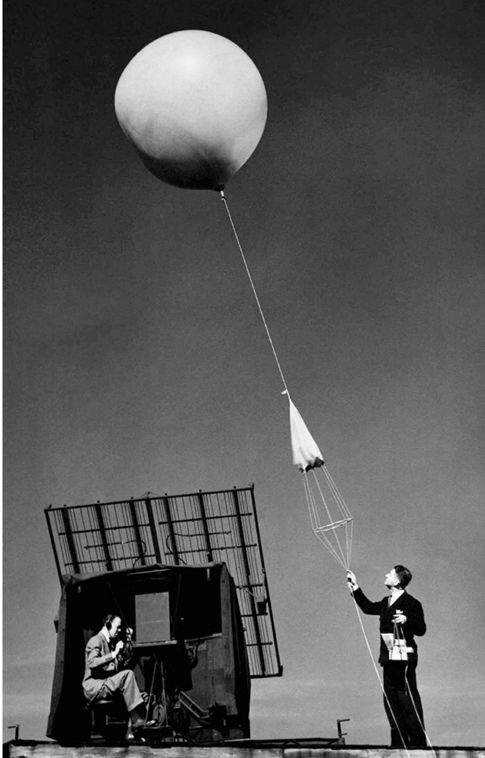
FIGURE 2. A RADIOSONDE READY TO BE LAUNCHED , circa 1940. The expendable instrument package, attached to a sounding balloon, measured the vertical profiles of atmospheric variables such as temperature, pressure, and humidity as the balloon rose from the surface to the stratosphere. Along the way, a radio transmitter in the package sent the data to a ground receiver. (Image from the National Archives and Records Administration RG-27, MD 27-G-10-16-1.)
