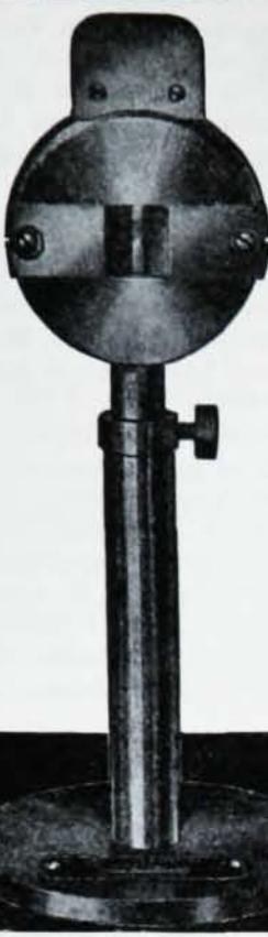
For many years the thermopile has been the accepted instrument for measuring Radiant Heat from Radiant Heaters at the American Gas Association Testing Laboratory in Cleveland, Ohio. Since 1930, when Vandaveer first described his work in this field,\* an Eppley thermopile has been used for this purpose in hundreds of tests and the results have been consistent and accurate to within 1 percent.
