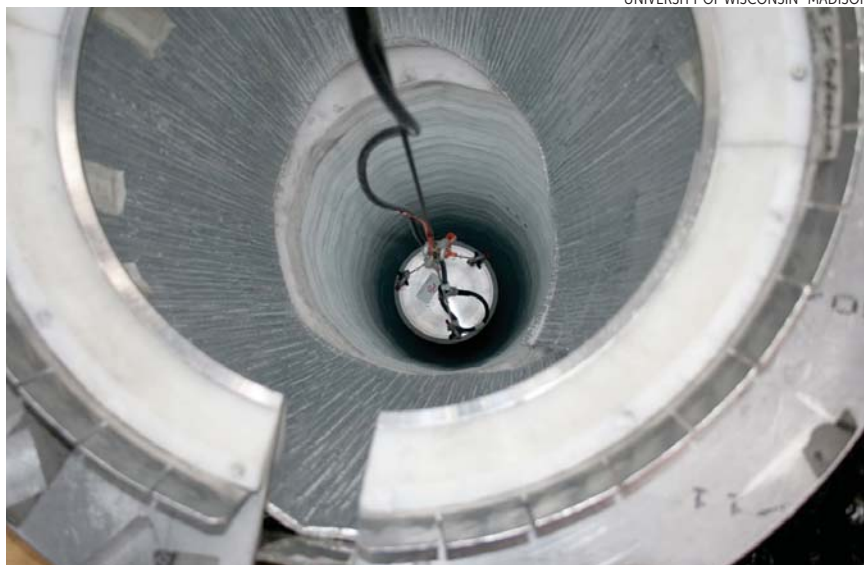
THE SODIUM IODIDE DETECTORS FOR THE DM-ICE EXPERIMENT are lowered into the Antarctic ice in 2010. DM-Ice will now use an improved set of detectors at a South Korean underground laboratory.
