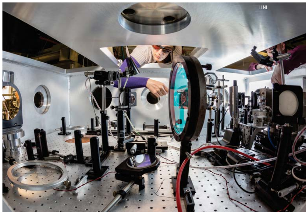
FÉLICIE ALBERT (center) and Bradley Pollock (right) prepare to do experiments with a betatron. The tabletop synchrotron produces femtosecond x-ray pulses and “is a good tool to probe dense plasmas,” Albert says. It took her several tries to win discretionary funding for the project at Lawrence Livermore National Laboratory.
