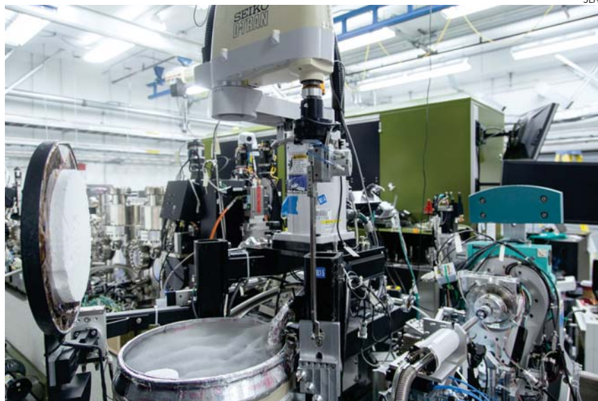
A HIGHLY AUTOMATED, ROBOTIC X-RAY CRYSTALLOGRAPHY SYSTEM at SLAC's Linac Coherent Light Source x-ray laser. The metal drum at the lower left contains liquid nitrogen for cooling crystallized samples. This setup was used to explore the molecular machinery involved in brain signaling in atomic-scale detail.
