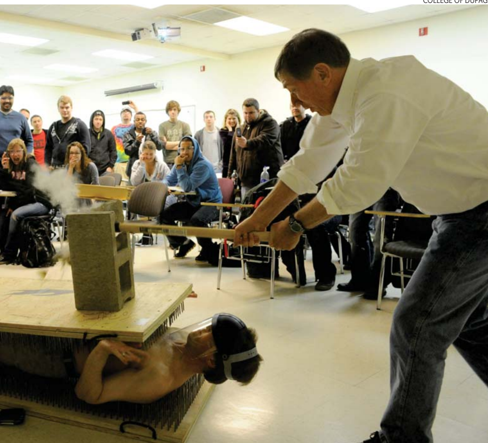
TO DEMONSTRATE KINETIC ENERGY AND INERTIA , Tom Carter breaks a cinder block over his brave colleague, Dave Fazzini. Most of the hammer's kinetic energy is absorbed in an inelastic collision with the block, the inertia of which saves the sandwiched professor from the nails in the upper board. The demonstration is for a class in conceptual physics that Fazzini teaches at the College of DuPage in Illinois.
