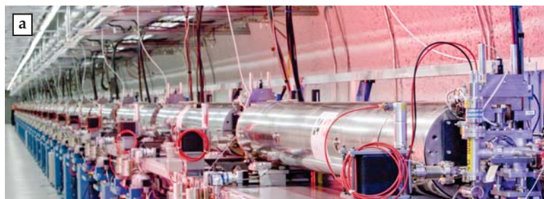
Figure 2. The 132-m undulator consisting of 33 individual segments (a) is the heart of the Linac Coherent Light Source. (b) This illustration shows the electrons' sinusoidal path (red wavy line) in the magnetic field of the undulator's array of permanent magnets with alternating north and south poles. The yellow arrow indicates the emitted photons. The x rays emitted by different electrons when they first enter the undulator are not coherent (lower left). In self-amplified spontaneous emission, the electrons interact with their own emissions and self-organize into microbunches (upper right) that wiggle synchronously to produce a coherent x-ray laser pulse. (Photo courtesy of SLAC.)
