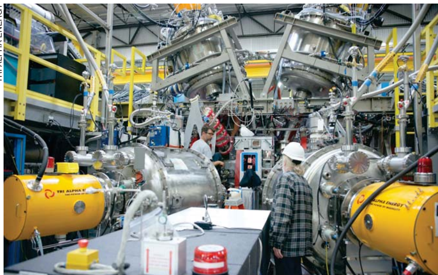
Tri Alpha Energy says it has produced a stable plasma in its C2U experimental device. Shown here are the accelerators that supply the beams of particles to help sustain the plasma.
