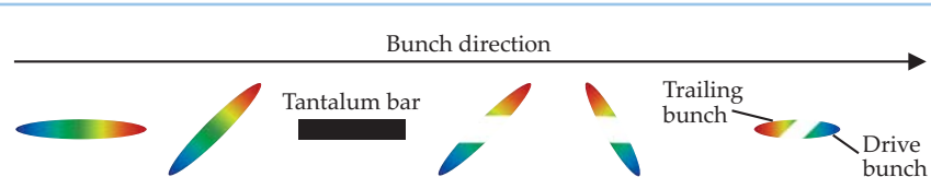
Figure 2. Two bunches from one. An electron bunch from the SLAC linear accelerator is dispersed according to its energy—here, the high-energy end of the bunch is shown in red and the low-energy end in blue. The bunch is then allowed to collide with a thin tantalum bar, which scatters the middle portion of the bunch out of the beam. (Adapted from ref. 1.)
