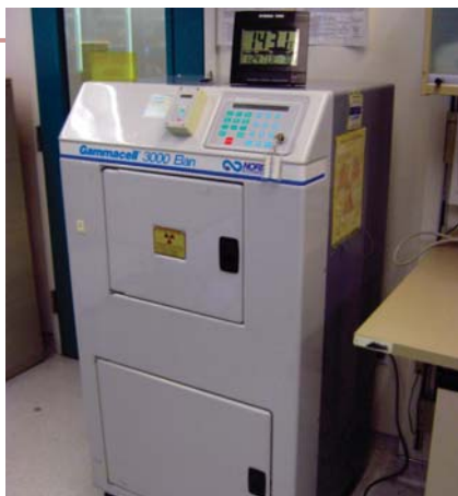
A self-contained irradiator in a medical facility. About 1100 irradiators, nearly all containing cesium-137, are used in US hospitals, blood banks, and universities for research and for treatment of blood.
