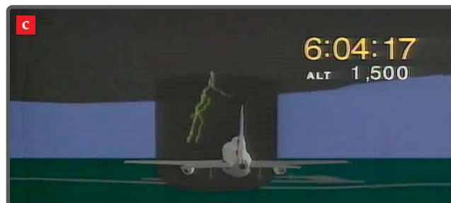
Figure 2. Still frames from three computer-generated movies re-create the weather conditions on 2 August 1985, during Delta flight 191's ill-fated approach to Dallas/Fort Worth International Airport. (a) A frame from a movie generated with ground-based radar data shows the location of storm clouds (gray) at 6:04:00pm and the aircraft's flight track up to that time. The white curve shows the flight track; each mark is labeled with a two-digit time stamp and the plane's altitude in feet. (b) A still from a second movie shows the aircraft-mounted radar
