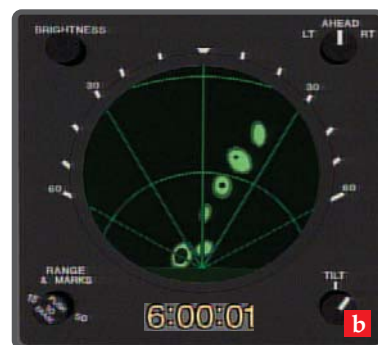
Figure 2. Still frames from three computer-generated movies re-create the weather conditions on 2 August 1985, during Delta flight 191's ill-fated approach to Dallas/Fort Worth International Airport. (a) A frame from a movie generated with ground-based radar data shows the location of storm clouds (gray) at 6:04:00pm and the aircraft's flight track up to that time. The white curve shows the flight track; each mark is labeled with a two-digit time stamp and the plane's altitude in feet. (b) A still from a second movie shows the aircraft-mounted radar
