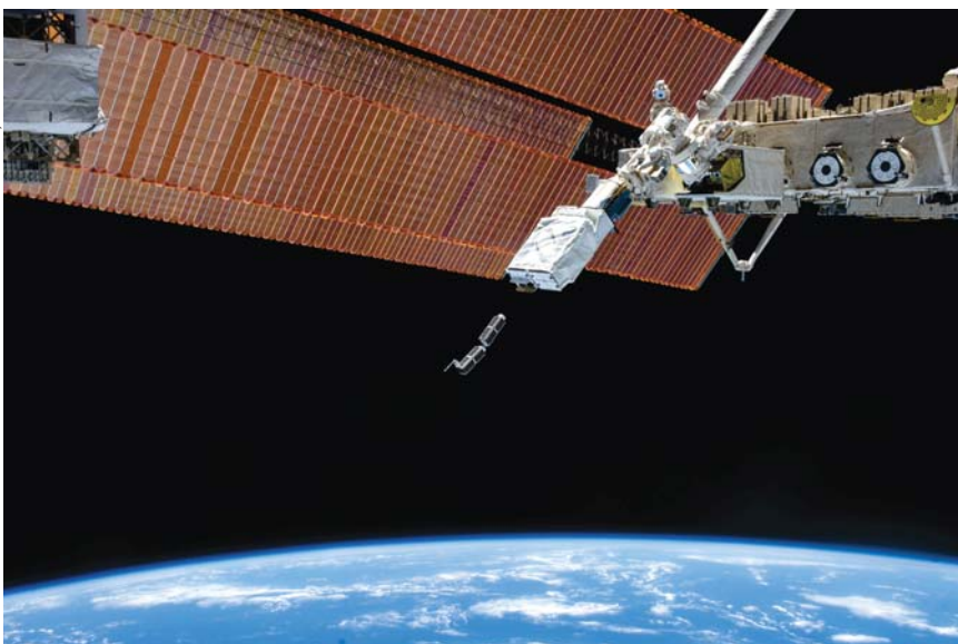
Two Planet Labs satellites being released from the International Space Station in February 2014; the solar panels open a day or so after release, as part of a remote commissioning process.
