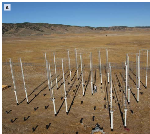
Figure 2. This bioinspired vertical-axis wind turbine (VAWT) farm (a) is located at Caltech's Field Laboratory for Optimized Wind Energy (FLOWE). There, arrays of up to 24 commercially available VAWTs are being tested in various configurations to study aerodynamic interactions and power generation. Scale is indicated by the author, who is standing in the center of the array. Video showing the turbines in operation is available at http://www.youtube.com/watch?v=cZu-4Plk_5A . (b) Shown here are measurements of footprint power density for 18-VAWT arrays at FLOWE. Open circles indicate direct measurements; filled circles show an extrapolation to an infinite VAWT array. The dashed range indicates performance with modern horizontal-axis wind turbines (HAWTs).
