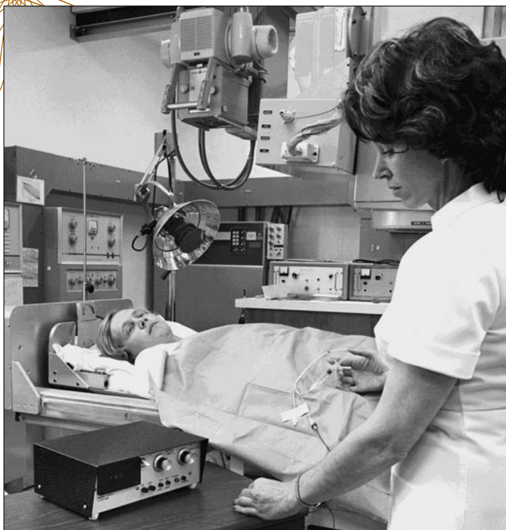
Figure 4. While demonstrating the thermodilution cardiac computer he designed to measure blood flow from the heart, master's of scientific instrumentation student Michael Buchin is injected with saline solution in a Santa Barbara hospital. (Photograph from 1974; courtesy of the Department of Special Collections, Davidson Library, UCSB.)
