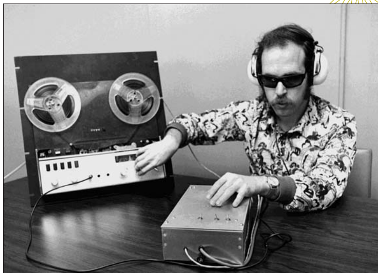
Figure 3. This tactile audio system was designed for blind audiophiles by students in the University of California, Santa Barbara, master's of scientific instrumentation program. Instead of having a visual meter for sound levels, it had metal pins representing Braille numbers. Here UCSB undergraduate Joe Renzi uses the device. (Photograph from 1975; courtesy of the Department of Special Collections, Davidson Library, UCSB.)
