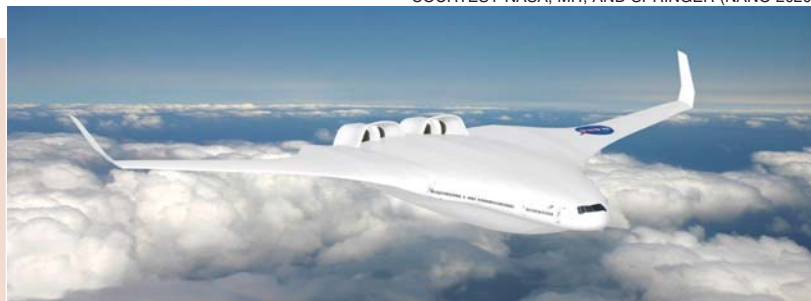
A passenger plane as conceptualized by researchers at MIT and NASA would exploit nanomaterials to cut weight, monitor performance to reduce emissions and improve safety, resist ice accretion, and change aerodynamic properties based on atmospheric conditions.
