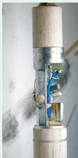
Figure 2. The apparatus for resonant ultrasound spectroscopy 1 contains two transducers 1.5 mm in diameter, which weakly couple to a crystal to probe its vibrational resonances. Balsa wood provides vibrational isolation over a broad temperature range.
