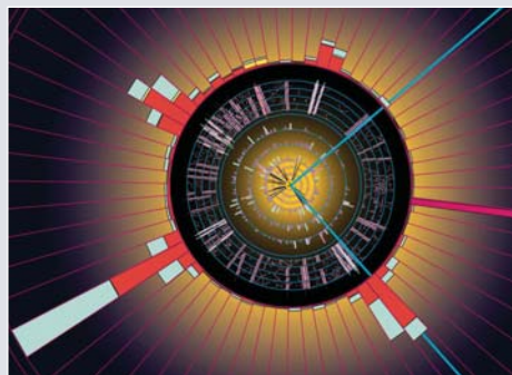
Figure 3. Beam's-eye view of a top-antitop quark pair created at the center of the Tevatron's D0 detector. One top quark decays to a W boson plus a bottom ( b ) quark, and that W promptly decays to a muon plus a neutrino. The other top quark also decays to W + b , but that W decays into two quarks that emerge as jets of hadrons at 8 and 10 o'clock. The lengths of the histogram bars around the cylindrical detector represent energy deposited by jets in azimuthal calorimeter segments surrounding the detector's inner tracking layers. The isolated blue line at 2 o'clock is the W -decay muon, and the jet encompassing the muon at 4 o'clock was generated by the decay of a b quark. The magenta bar at 3 o'clock indicates the missing energy and direction of the escaped neutrino.
