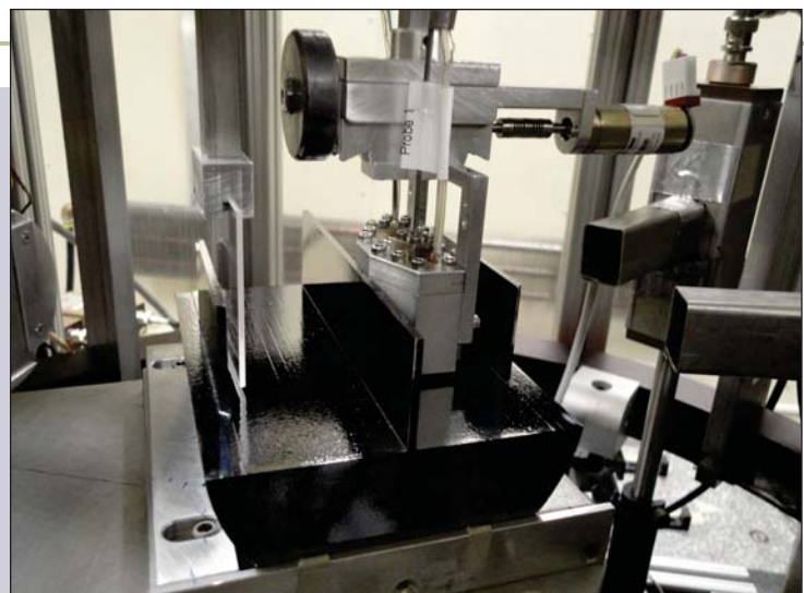
Figure 4. The neutron interferometer illustrated at left and pictured at right comprises three parallel blades carved from a single silicon crystal. Roughly 10 cm wide, it's used by NIST researchers to coherently split and recombine incident beams of slow neutrons. By rotating the interferometer about the incident-beam axis, one can detect a subtle gravitational phase shift that stems from the slight difference in height of the interferometer paths. Similarly, by detecting the phase shift that arises when a test sample (orange in the illustration) is placed in one of the interferometer paths, one can precisely determine the sample's neutron scattering amplitude. To achieve a high signal-to-noise ratio, the interferometer must be protected by multiple thermal and vibrational isolation enclosures. (Photo courtesy of Muhammad Arif.)
