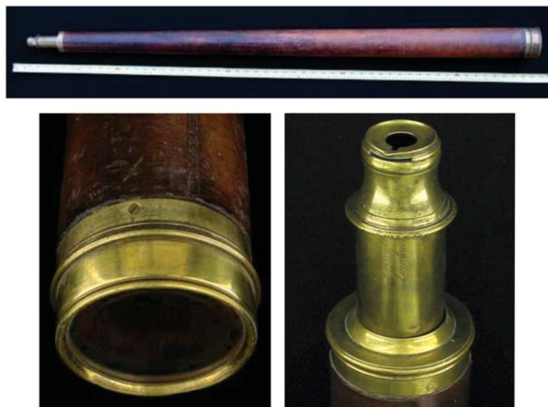
Figure 2. The 140-cm-long Dollond telescope used by Alexandre Koukarine during the 2012 transit of Venus, with close-ups of the lens housing and eyepiece.
