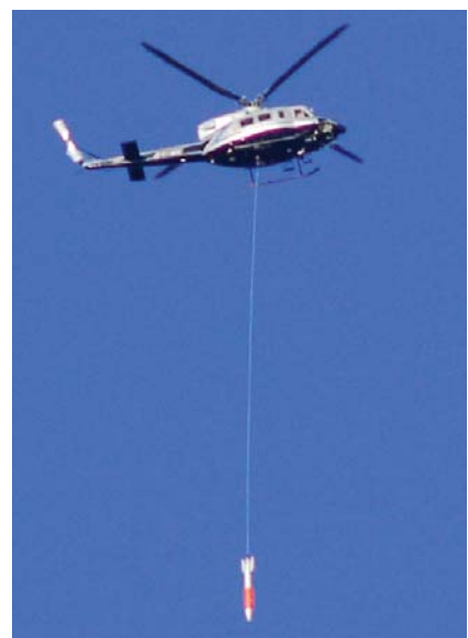
A replacement radar device for the modernized B-61 nuclear bomb was drop-tested from a helicopter in Nevada this summer.
