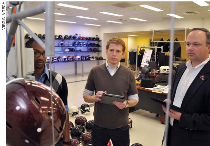
Helmet lab: From left, Ray Daniel, Steven Rowson, and Stefan Duma measure the effects of various applied linear and rotational forces on helmets and dummy heads.
