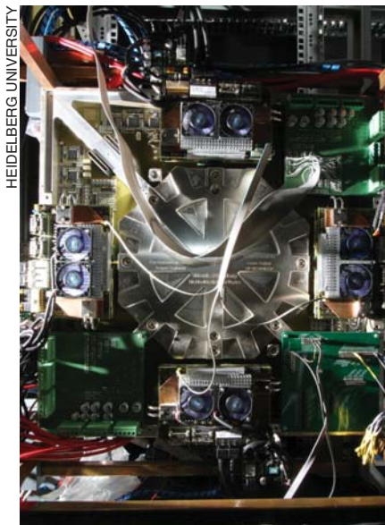
This neuromorphic computing system in Heidelberg mimics 200 000 neurons and 50 million synapses on a silicon wafer located behind the central octagonal aluminum plate. Field-programmable gate arrays configure the network and send and read input and output data.
