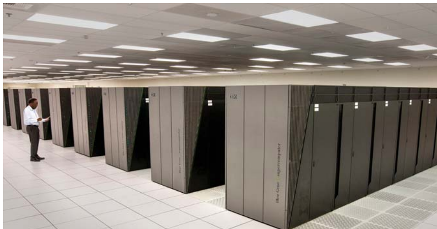
Sequoia, an IBM Blue Gene/Q system at Lawrence Livermore National Laboratory, was ranked third in the world in computing performance in June by the widely recognized Top 500 supercomputer sites listing ( www.top500.org ); it achieved 17.17 petaflops. Consuming 7.8 MW and delivering 2 gigaflops/W, Sequoia is also one of the most energy efficient of the top computers.
