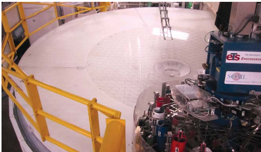
Casting the primary mirror (outer 8.4-m dish) and tertiary mirror (inner 5-m dish) out of a single piece of glass saves money and reduces alignment problems for the Large Synoptic Survey Telescope.
