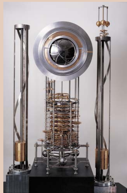
This 2.4-meter prototype to test some mechanisms for a larger 10 000-year clock chimed at the turn of the last millennium and now stands in the London Science Museum. (Rolfe Horne, courtesy of The Long Now Foundation, http://www.longnow.org .)
