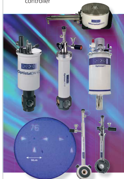
Microscope image of masked InGaN quantum dot sample cooled by a MicrostatHires2 . A 1 µm hole can be seen at the center of the three arrows labeled 76. Courtesy of Prof. Robert Taylor, Clarendon Laboratory, Oxford University.
