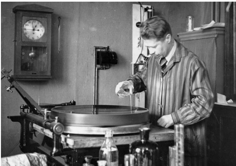
Yrjö Väisälä in the physics department's machine shop at the University of Turku, Finland, in 1934. He is silversmithing the primary mirror of an anastigmatic telescope. (Courtesy of the University of Turku Central Archives.)
