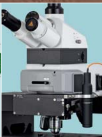
Automated Raman-AFM system alpha500 with attached sensor for profilometry
