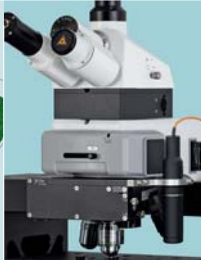
Automated Raman-AFM system alpha500 with attached sensor for profilometry
