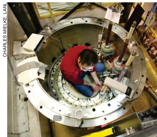
This nondestructive magnet at Los Alamos National Laboratory last summer achieved a record pulse of 97.4 T. The lab plans to offer 92-T pulses to users soon.
