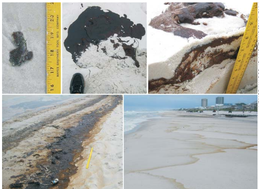
In a research project funded by NSF’s Rapid Response Research program, Ping Yang and others at the University of South Florida identified multiple forms of oil contamination along Alabama and northern Florida beaches. Clockwise from upper left, the forms are tar ball, tar patty, tar cake, oil stain, and oil sheet. Measuring stick is one yard long.
