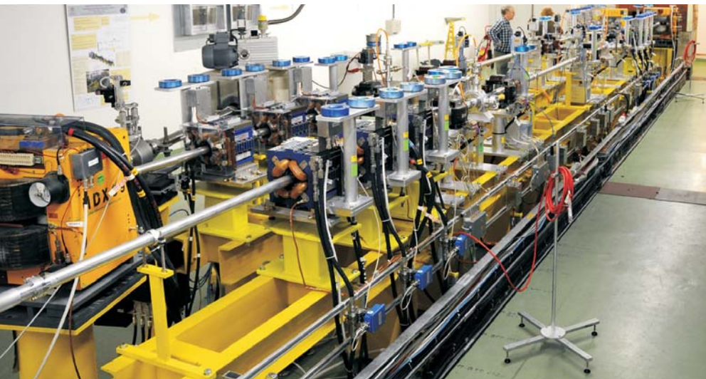
Feasibility tests for the Compact Linear Collider are in progress at CERN's 17-meter-long two-beam test stand. A high-intensity, short-pulsed drive beam (closer beam) feeds the main beam through RF power extraction.
