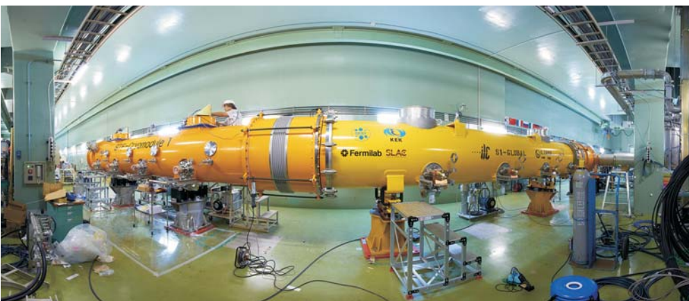
Tests on a cryomodule containing eight superconducting cavities are getting under way. The tests are intended to show that the International Linear Collider's acceleration technology works, and that it works with parts fit together from around the world. The ILC would have more than 1000 such cryomodules.
