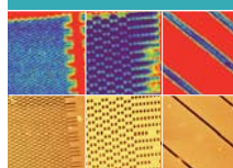
Raman stress and AFM topography images recorded automatically at three different areas of a Si-device.
