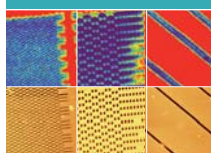
Raman stress and AFM topography images recorded automated at three different areas of a Si-device.
