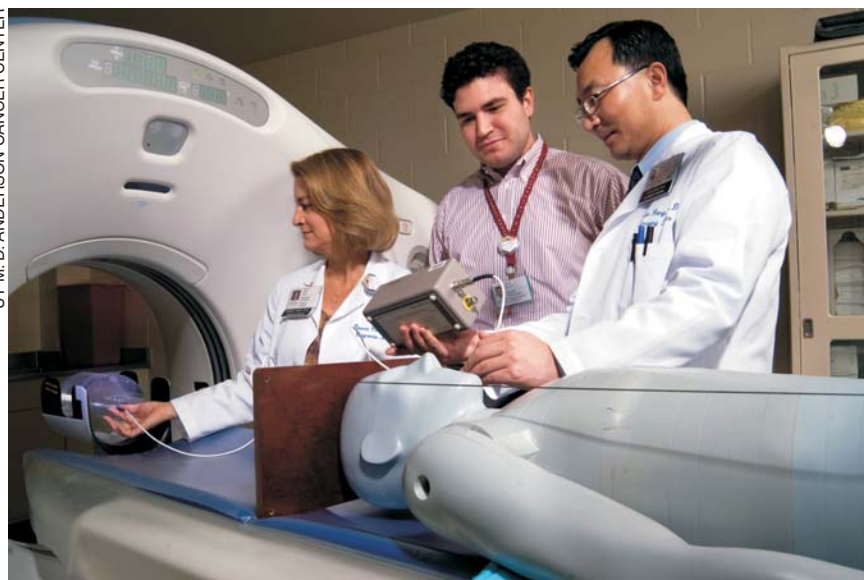
A human phantom is used for radiation dosimetry point measurements by medical physicists Dianna Cody and John Rong (right) and physics technologist David Zamora (middle) at the University of Texas's M. D. Anderson Cancer Center.
