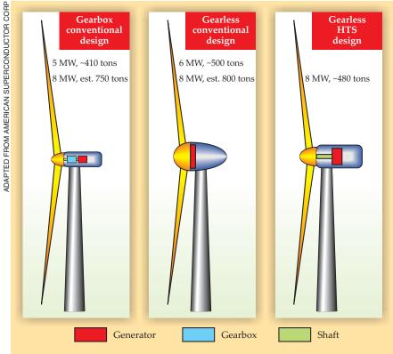
Lightweight, superconducting generators will make possible 8- to 10-MW wind turbines (right) at a fraction of the weight and size that geared (left) and gearless (center) conventional copper-wire generators would have to be. (Adapted from American Superconductor Corp.)
