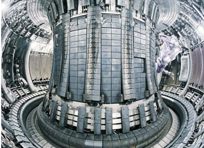
The thousands of carbon tiles lining the plasma-facing wall inside the vacuum vessel of the Joint European Torus are being replaced using a remote-controlled slave arm.
