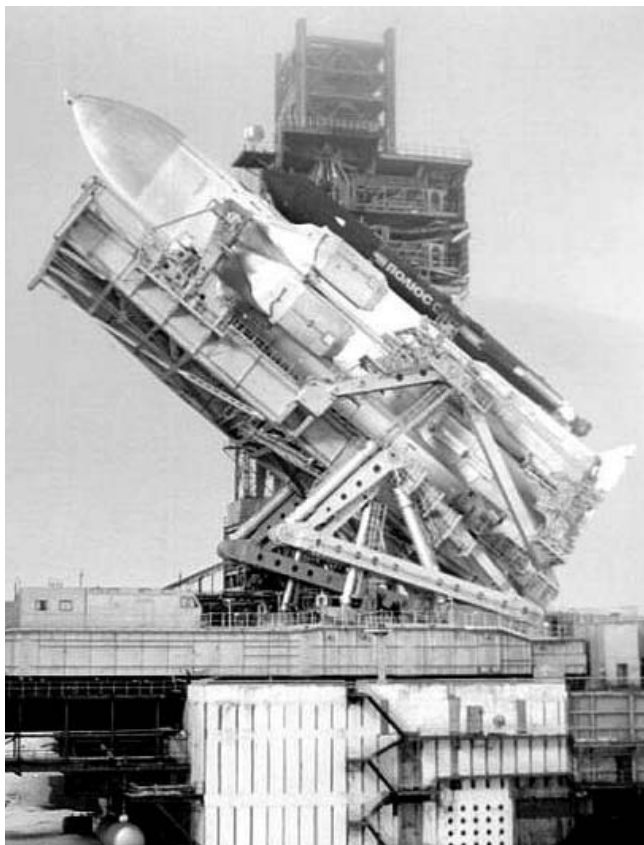
Polyus , a 37-meter-long Soviet spacecraft carrying a missile-defense test bed, is the dark vehicle strapped atop an Energia rocket on the launch pad. It was launched in May 1987 but failed to reach orbit.
