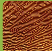
MFM Image of Garnet Single Crystal
