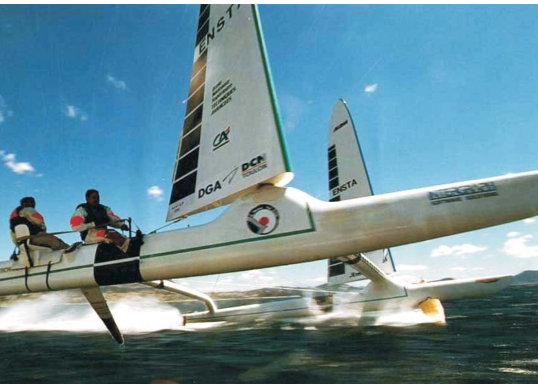
Figure 6. A hydrofoil sailboat with solid, winglike sails, moving at about twice the wind speed with the wind abeam—that is, blowing from the side. (Copyright École Nationale Supérieure de Techniques Avancées.)
