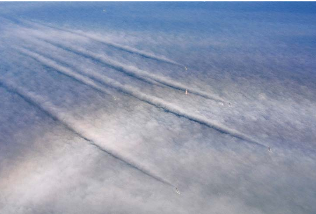
Figure 3. Sailtops form vortices visible in fog. The boats were participating in the 2001–02 Volvo Ocean Race off Cape Town, South Africa. (Photo copyright Daniel Forster, used with permission.)
