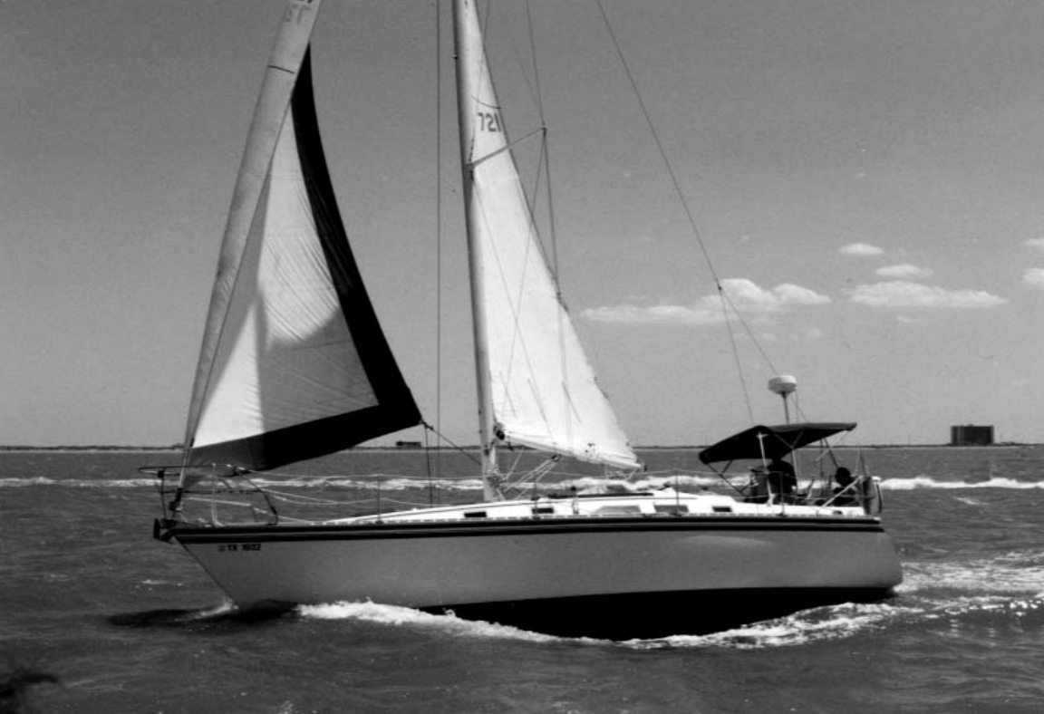
Figure 4. Moving at hull speed, a sailboat generates a bow wave whose wave-length just equals the length of the boat's water line. The wave crests at bow and stern, with a single well-formed trough in between. (Photo by Greg Green, used with permission.)
