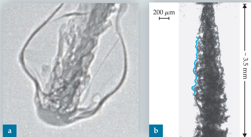
Figure 4. Imaging the liquid core in an atomizing spray. (a) The structure of the leading edge of an impinging spray (entering from the upper right) is instantaneously captured using single-shot short-pulsed x-ray phase-contrast imaging with 300-ns resolution. The complex structure of the dense spray arises because of turbulence in the flow. The large balloonlike structure results from the initial ejection of static liquid trapped in the flow cavity, commonly called the sac volume. (Adapted from ref. 18.) (b) The near field of an atomizing diesel fuel spray is captured in this ballistic image taken with high spatial (25 \mu\text{m} ) and temporal (3 ps)
