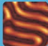
MFM Image of Garnet Single Crystal at 1.9K
