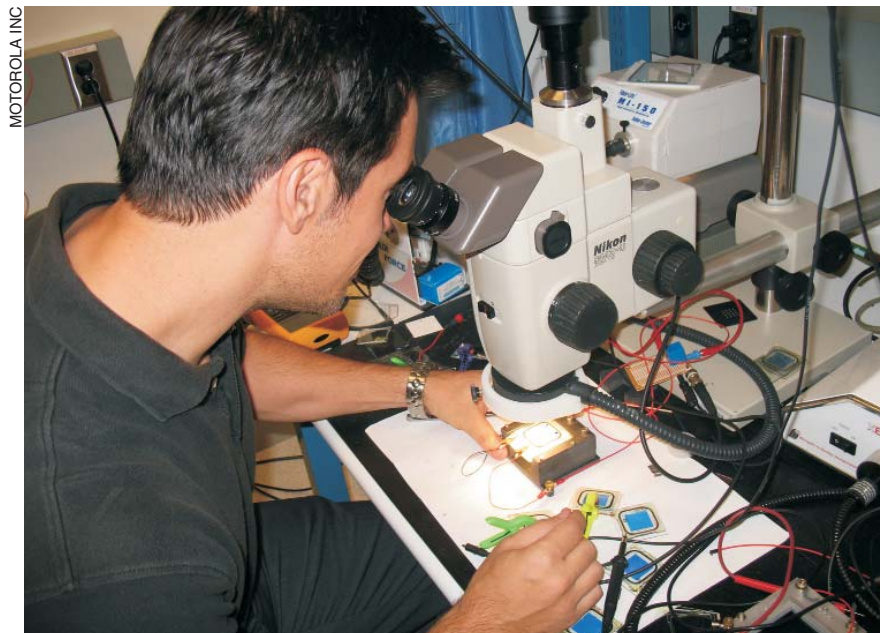
The nano-emissive display glass sample shown here undergoing electronic tests by Motorola engineer Michael Johnson incorporates thermally grown carbon nanotubes as electrodes and is expected to compete with the cost and picture quality of LCD TVs.
