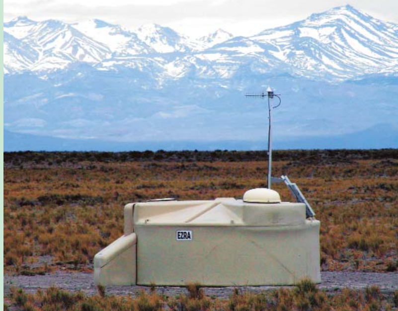
Figure 2. One of the Auger ground array's 1600 water-Cherenkov detectors, with the Andes looming on the western horizon. Each detector holds 10 tons of water monitored by phototubes for Cherenkov light pulses. One can see the detector's battery pack (left), its north-facing solar panel, and its electronics dome topped by a communications mast.
