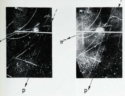
The first V particle identified at the Cosmotron appears above the sweeping field electrode in the center of the picture, at the point indicated by the arrow. Two stereo views are shown. The sweeping field electrode is actually closer to the camera than the sensitive region, and the tracks pass behind it, not through it.
