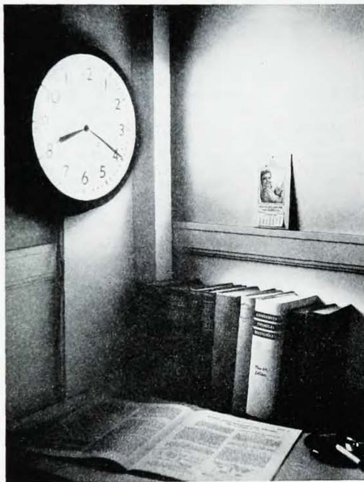
Fig. 9. Photograph of a clock and its surroundings. The light by which this photograph was taken was furnished by the electroluminescent dial with which the clock was provided.
