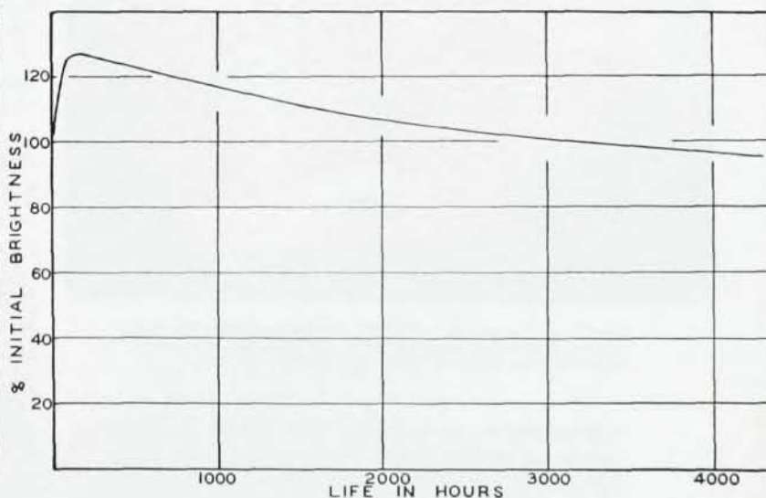
Fig. 7. Curve showing the variation of light output from a typical electroluminescent lamp as a function of operating time.
